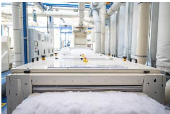
ANDRITZ textile recycling line based on tearing
